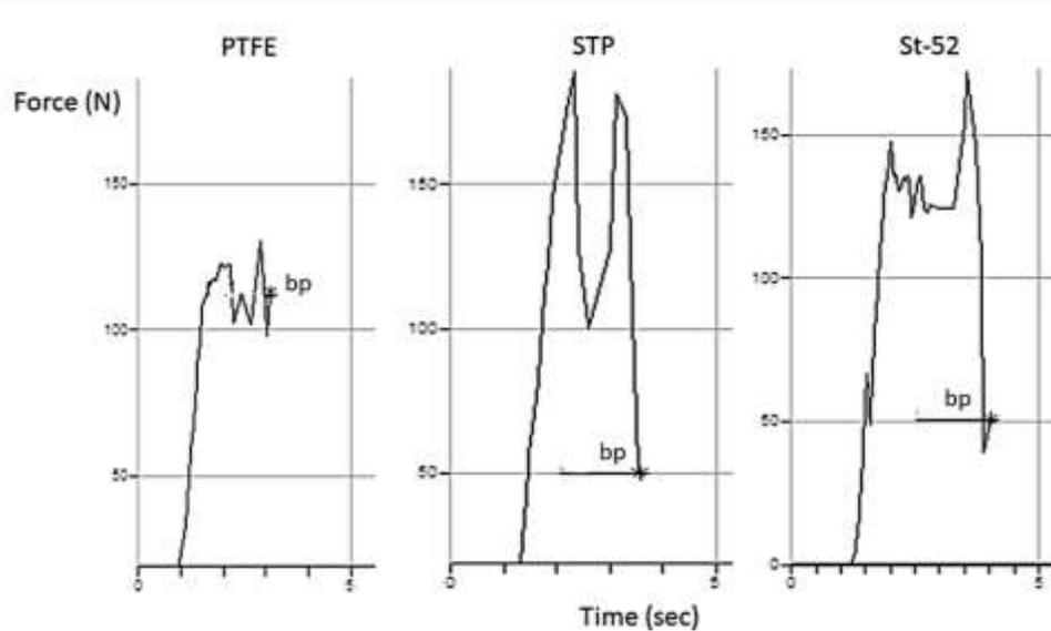
Figure 4. Variation of cutting force with time.
