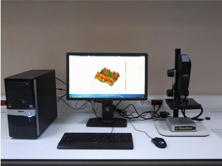
**Figure 3.** Optical Profilometer device.
