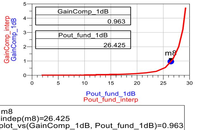
Fig. 11. Gain Compression versus 1dB
