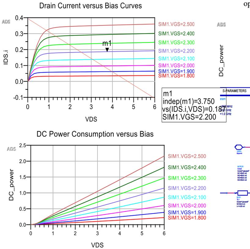
**Fig. 2.** DC biasing of the desired Transistor output characteristics
