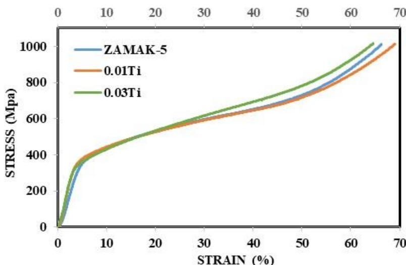
**Figure 6.** Stress-strain curves of the samples obtained by compression tests.
