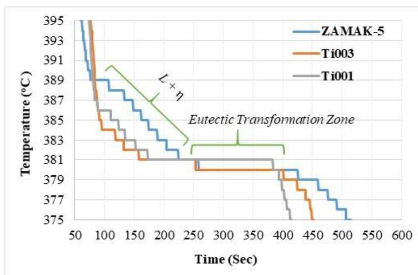
**Figure 3.** Cooling curves of the samples.
