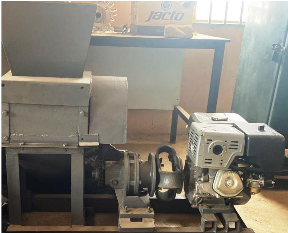
Figure 10. Front view of the developed shredder assembly.
