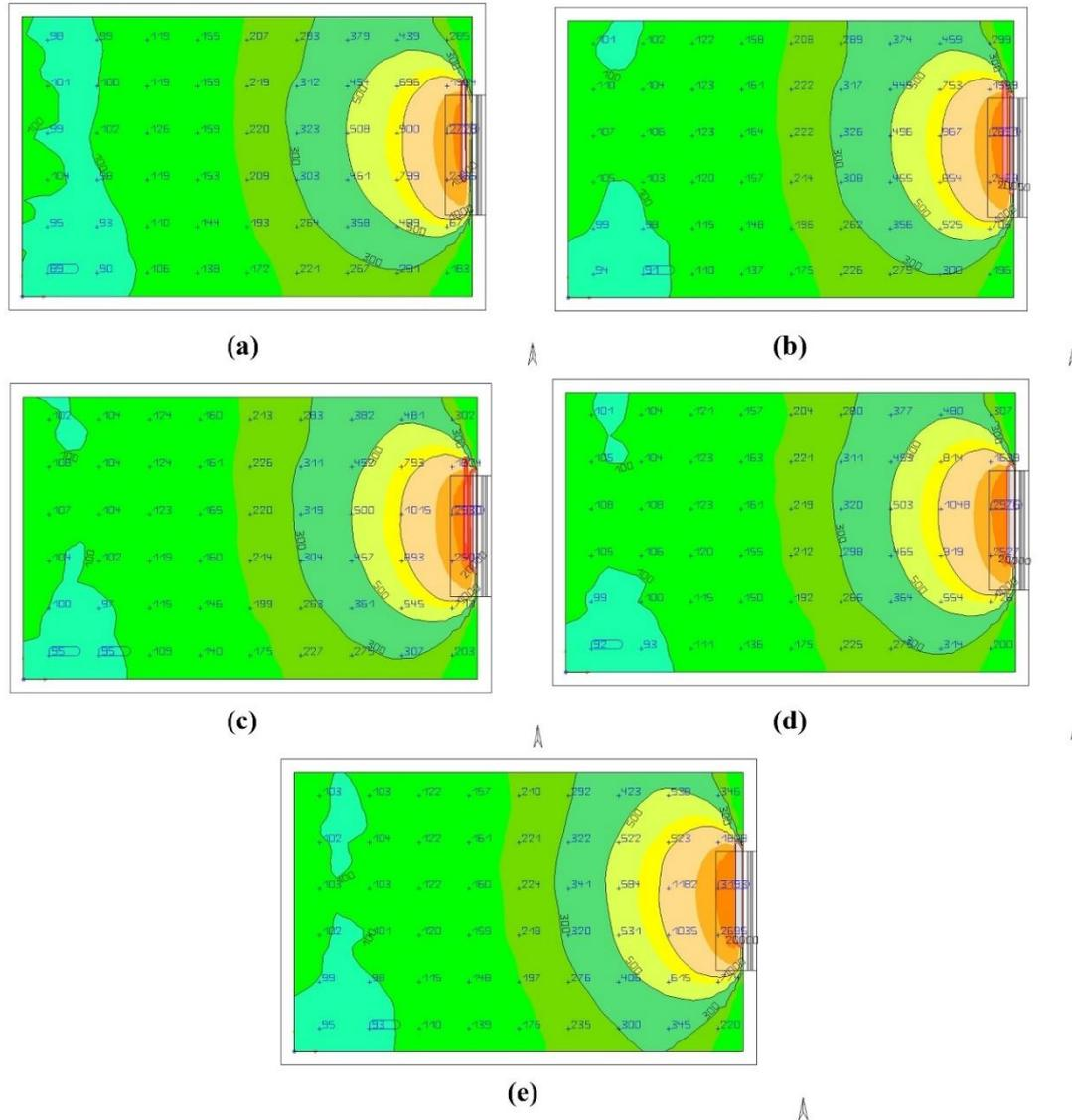
**Figure 9.** Light shelf height comparison. (a): Light shelf on 170 cm height. (b): Light shelf on 180 cm height. (c): Light shelf on 185 cm height. (d): Light shelf on 190 cm height. (e): Light shelf on 200 cm height.
