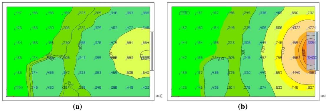
**Figure 18.** Comparison of no light shelf and with light shelf measurements (a): Without light shelf. (b): With light shelf.
