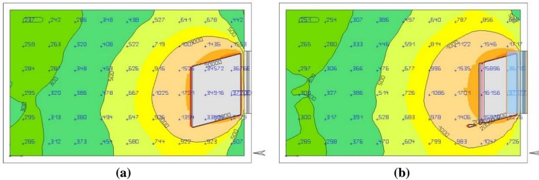
**Figure 20.** Comparison of no light shelf and with light shelf measurements (a): Without light shelf. (b): With light shelf.
