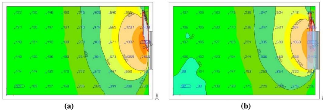
**Figure 21.** Comparison of no light shelf and with light shelf measurements (a): Without light shelf. (b): With light shelf.
