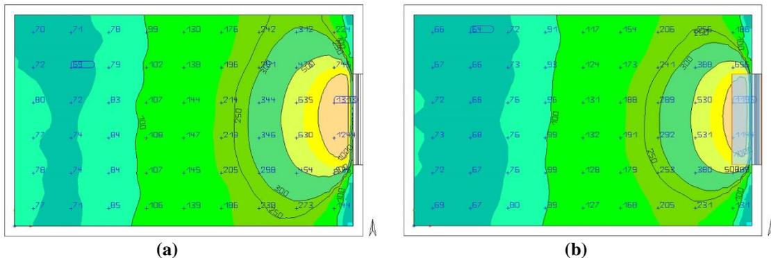
**Figure 23.** Comparison of no light shelf and with light shelf measurements (a): Without light shelf. (b): With light shelf.
