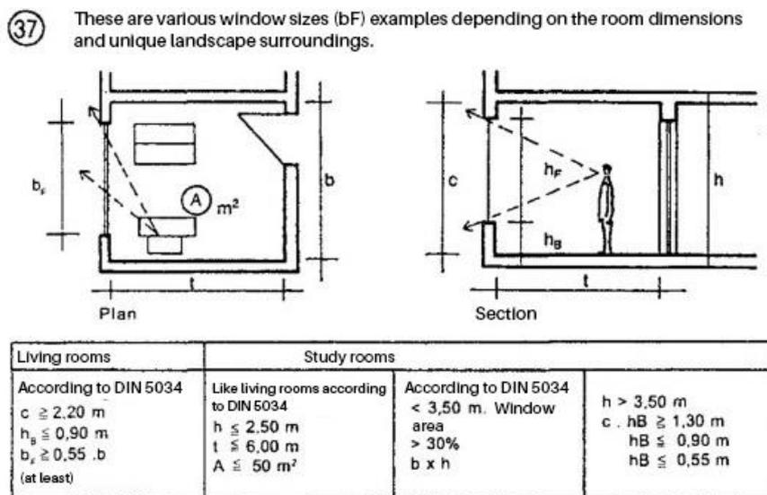
Figure 1. DIN5034 Window openings and room sizes are foreseen for different room dimensions [6].
