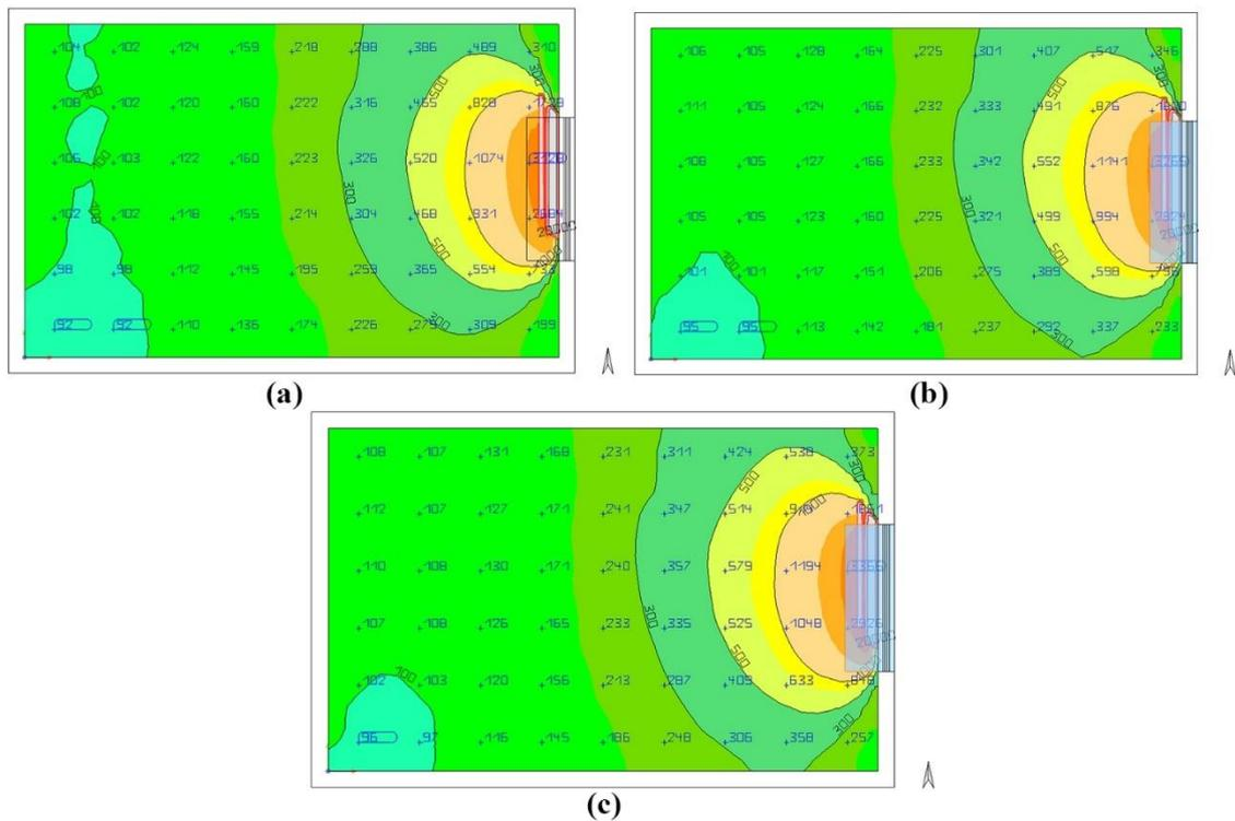
**Figure 7.** Comparison of light shelf reflection values (a): Reflection value of the light shelf on DiaLux software in default wooden material settings (0.15  $\rho$ ). (b): Reflection value of the wooden light shelf (0.50  $\rho$ ). (c): Reflection value of the composite light shelf material (0.80  $\rho$ ).
