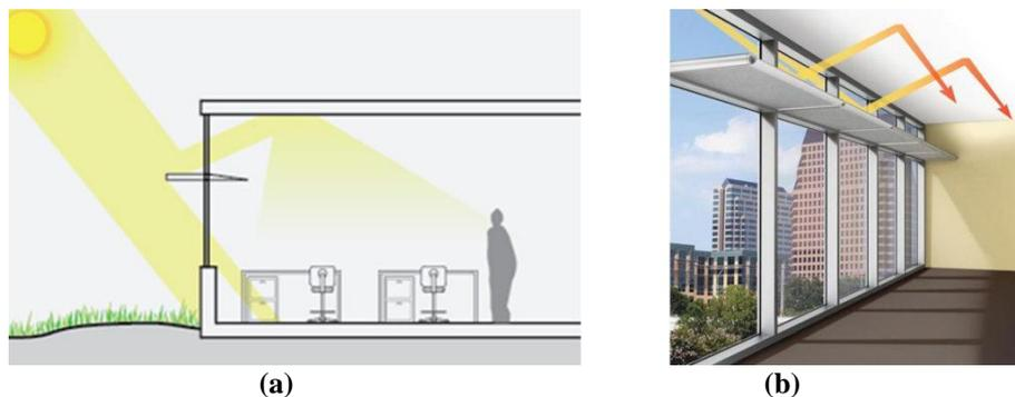
**Figure 2.** Access to the interior of light through light shelves [10]. (a): section, (b): 3d image
