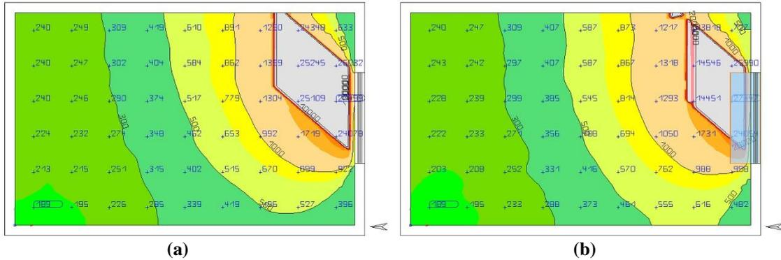
**Figure 22.** Comparison of no light shelf and with light shelf measurements (a): Without light shelf. (b): With light shelf.
