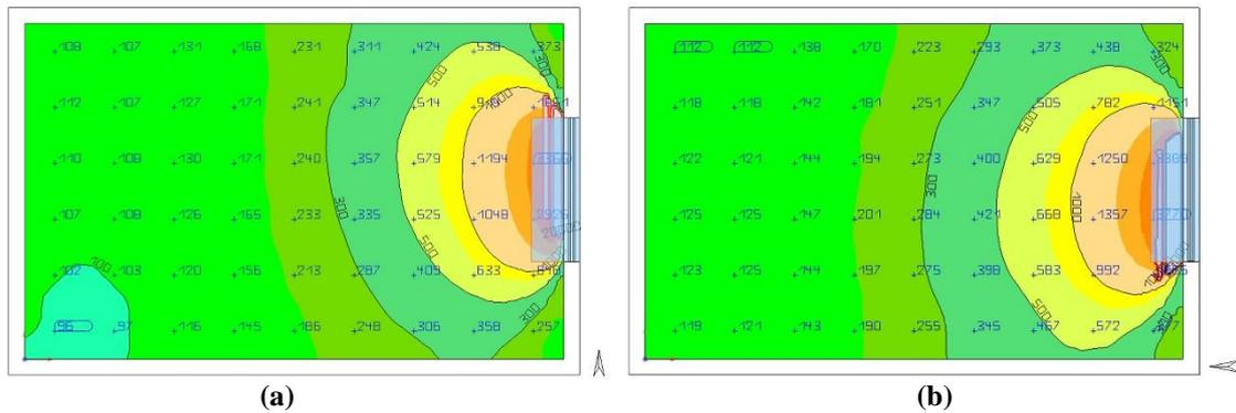
**Figure 8.** Daylight measurements made in different directions of room's opening (a): East direction. (b): South direction.
