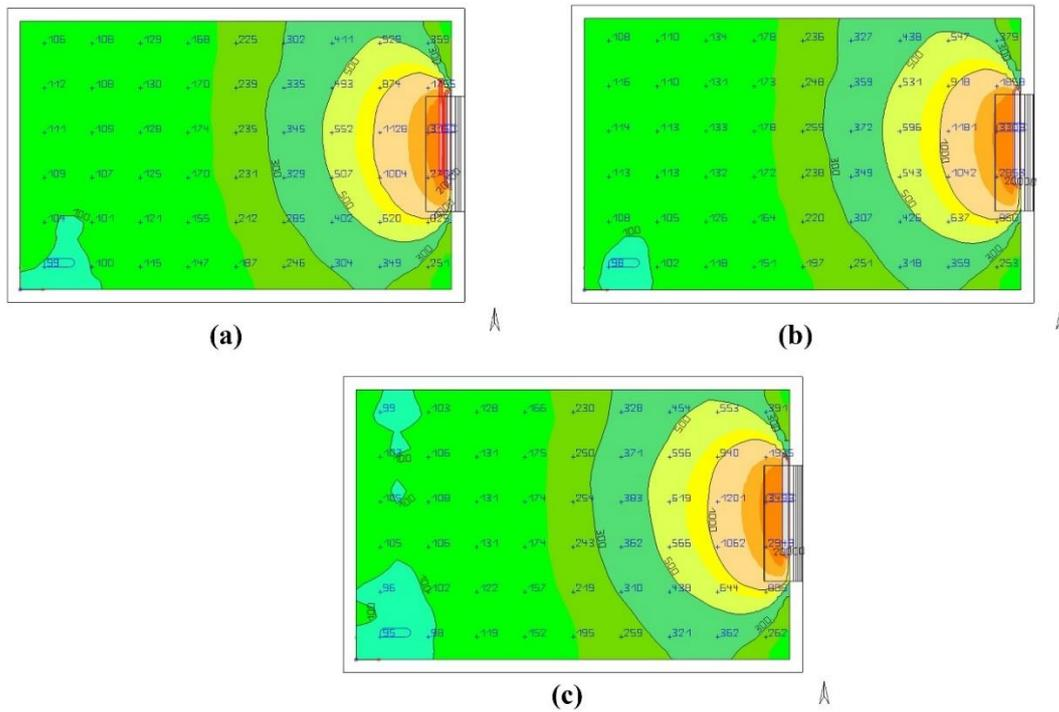
**Figure 10.** Light shelf slope comparison. (a): Light shelf's slope is 0°. (b): Light shelf's slope is 10°. (c): Light shelf's slope is 20°.
