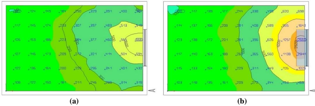
**Figure 19.** Comparison of no light shelf and with light shelf measurements (a): Without light shelf. (b): With light shelf
