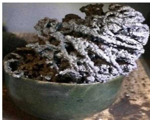
Figure 5: A sample of the catalyst Co-Fe=1:2 obtained sol-gel method with auto-burning.
