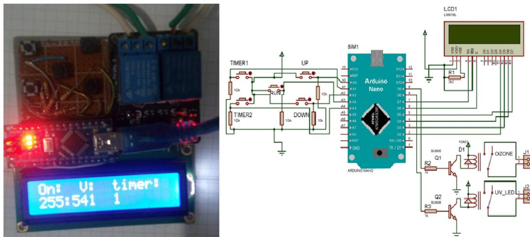
Figure 3. Digital timer circuit and its components.
