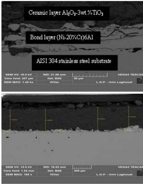
Figure 1. SEM micrographs of  $Al_2O_3/3wt.\%TiO_2$
