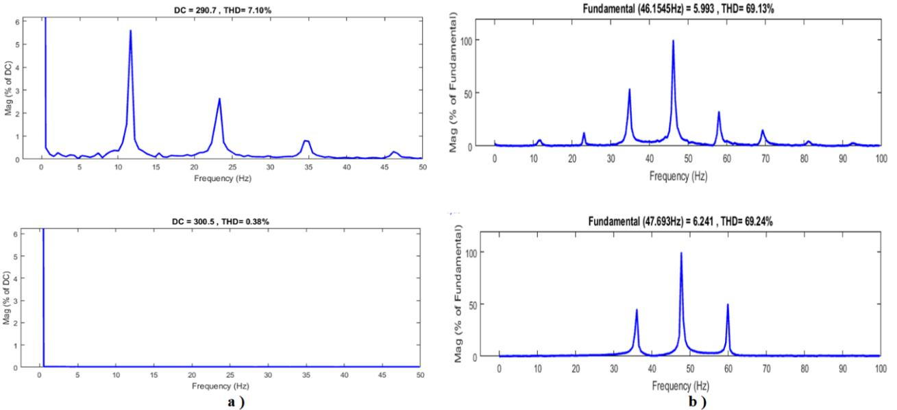
Figure 3. a) Motor speed FFT analysis and b) motor torque FFT analysis
