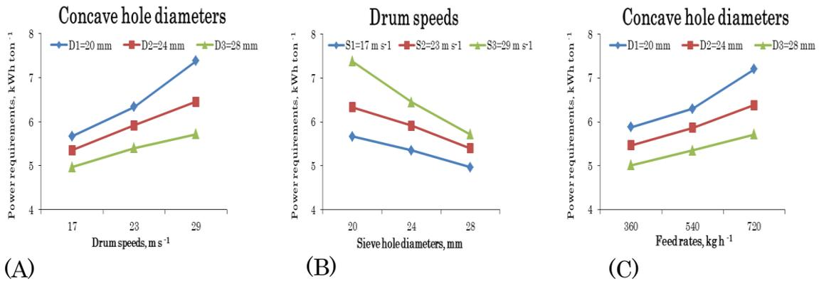
**Figure 7.** (A). Effect of drum speeds on the power requirements at concave hole diameters; (B) Effect of concave hole diameters on the power requirements at drum speeds; (C) Effect of feed rates on the power requirements at concave hole diameters.
