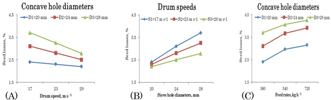
**Figure 5.** (A) Effect of drum speeds on seed losses at concave hole diameters; (B) Effect of concave hole diameters on seed losses at drum speeds; (C) Effect of feed rates on seed losses at concave hole diameters.
