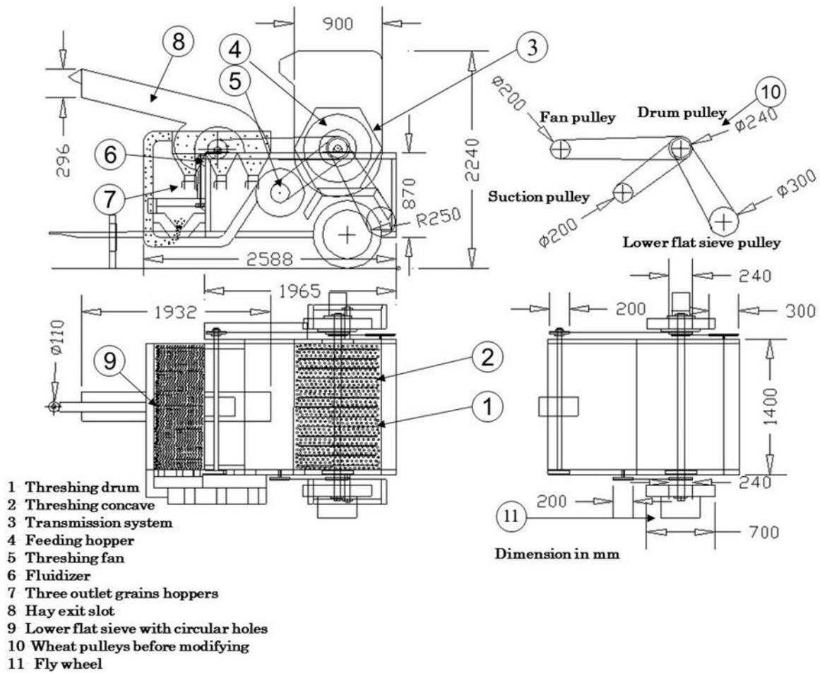
Figure 1. Threshing machine before modification.
