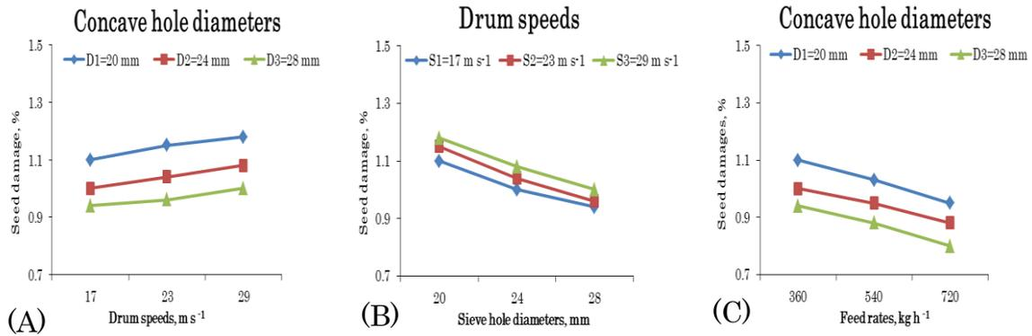
**Figure 6.** (A) Effect of drum speeds on seed damage at concave hole diameters; (B) Effect of concave hole diameters on seed damage at drum speeds (C) Effect of feed rates on seed damage at concave hole diameters.
