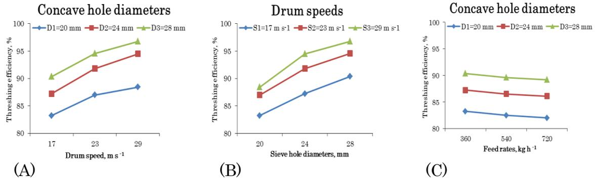
**Figure 4.** (A). Effect of drum speeds on threshing efficiency at concave hole diameters; (B). Effect of concave hole diameters on threshing efficiency at drum speeds; (C). Effect of feed rates on threshing efficiency at concave hole diameters.
