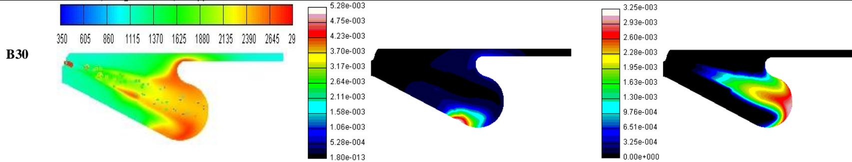
Figure 7 Variation of temperatures, NO and Soot fraction at 10 CA
