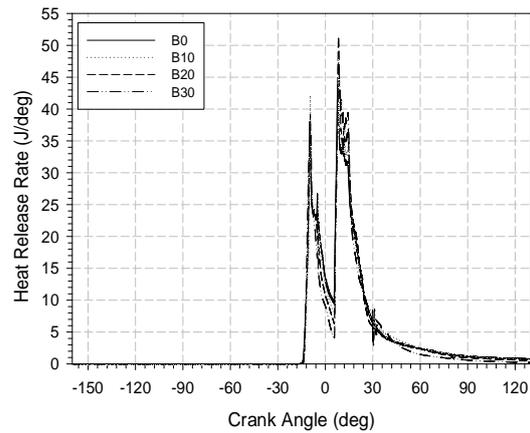
**Figure 3** Comparison of (a) the in-cylinder pressure, and (b) the heat release rate (HRR) for diesel-biodiesel blends
