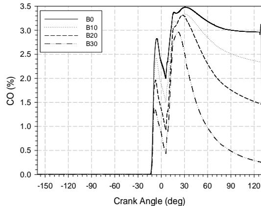
**Figure 5** In-cylinder CO emission histories with respect to crank angle for diesel-biodiesel blends
