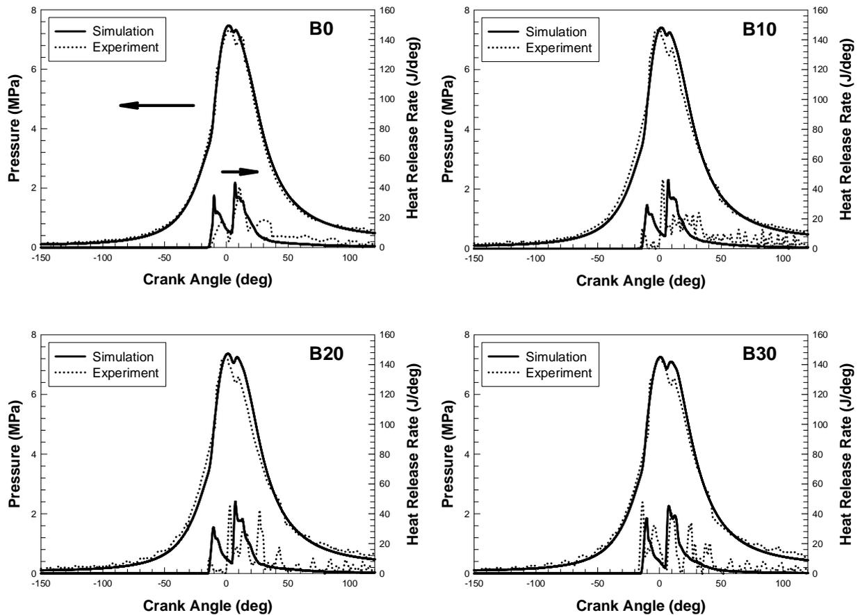
**Figure 2** Experimental and calculated in-cylinder pressure and heat release rates with respect to mixing ratios of biodiesel
