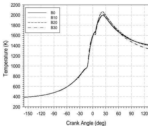
**Figure 4** In-cylinder average combustion temperature for fuels
