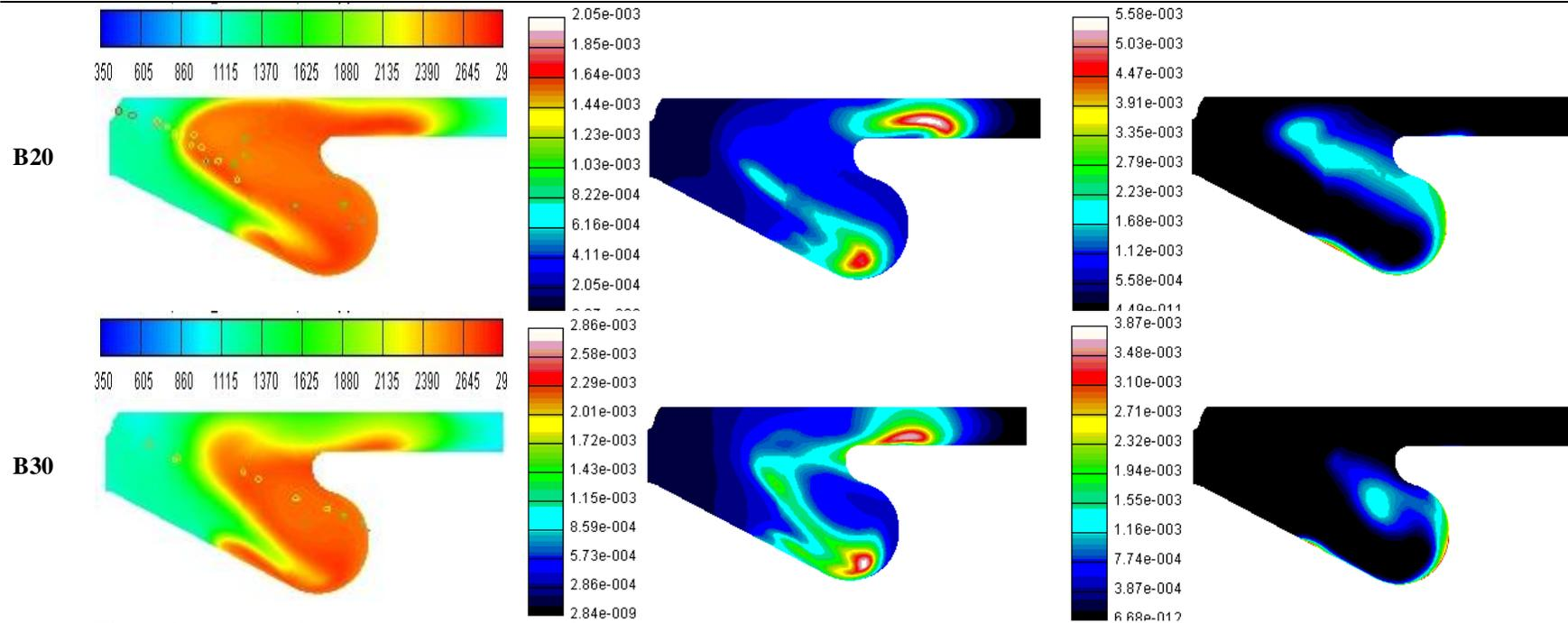
Figure 8 Variation of temperatures, NO and Soot fraction at 20 CA
