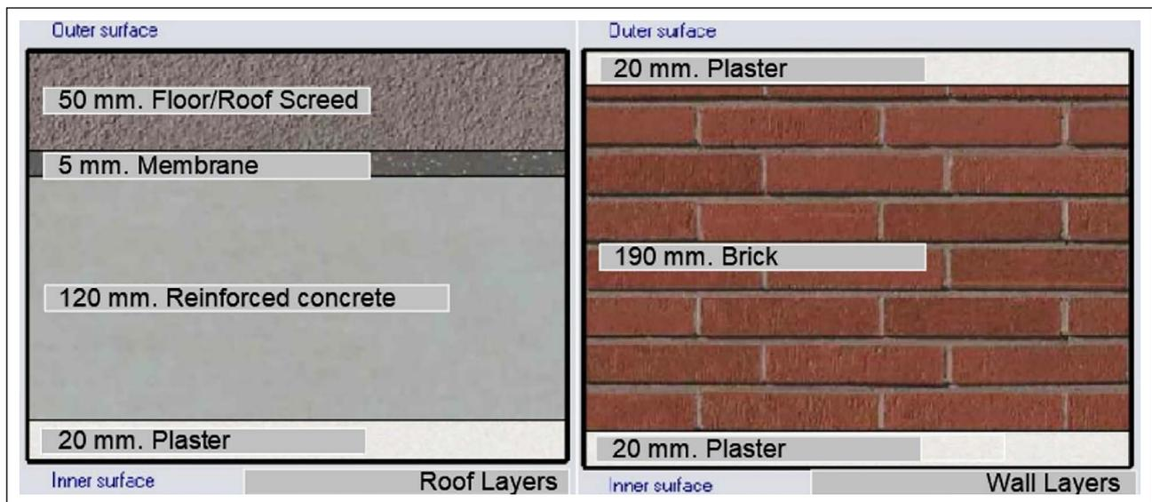
Figure 3. Layers of materials are used in the roof and walls.
