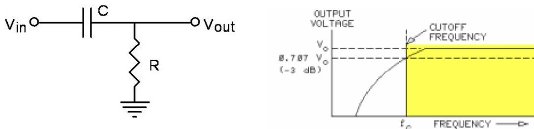
Figure-7 Analog RC Passive Highpass Filter and Its Frequency Response
