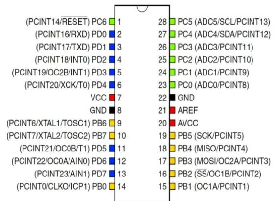
Figure-11 Atmel Atmega-328P
