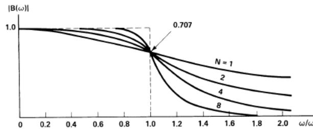
Figure-9 Butterworth Filter Frequency Response
