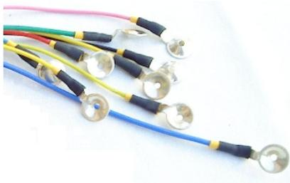
Figure-4 Metal disc electrodes
