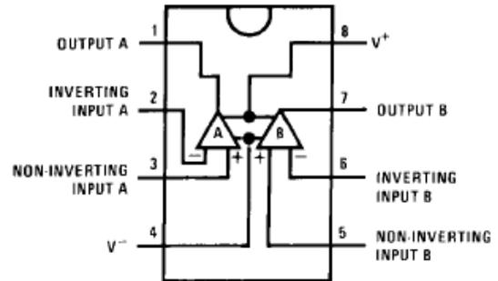
Figure-8 LF412 Pinout
