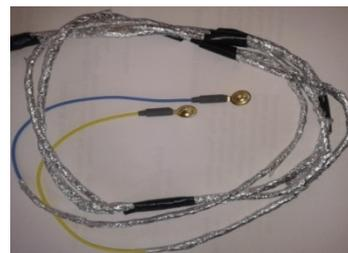
Figure-5 Isolated electrodes
