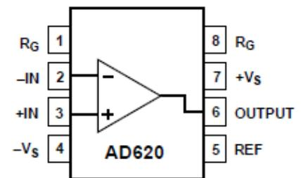
Figure-6 AD620 Pinout
