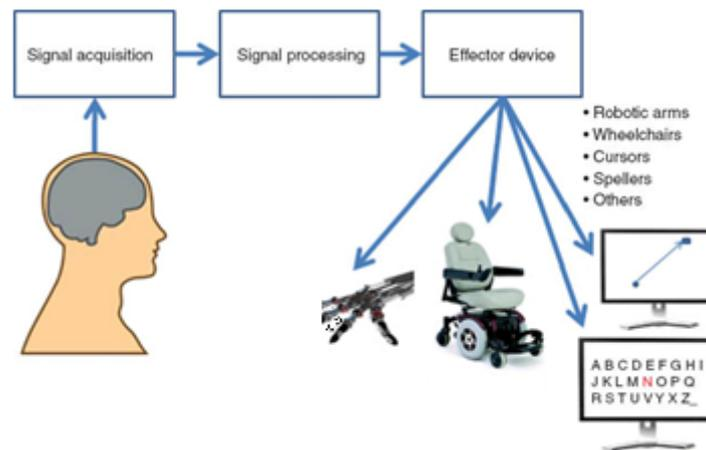
**Figure-1** The General Structure of BCI Systems
