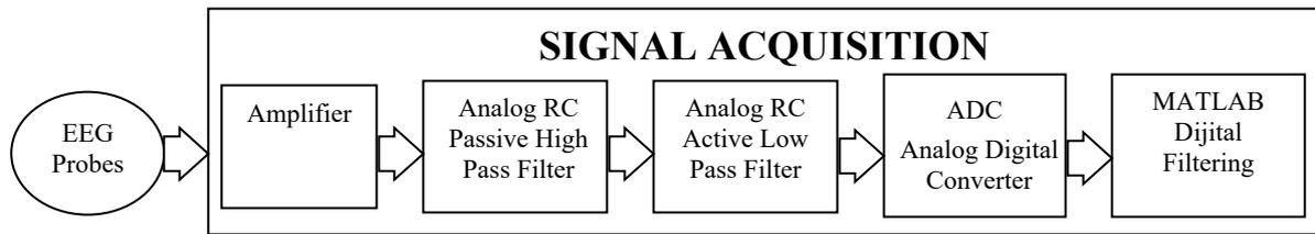
Figure-2 Block Diagram of The System
