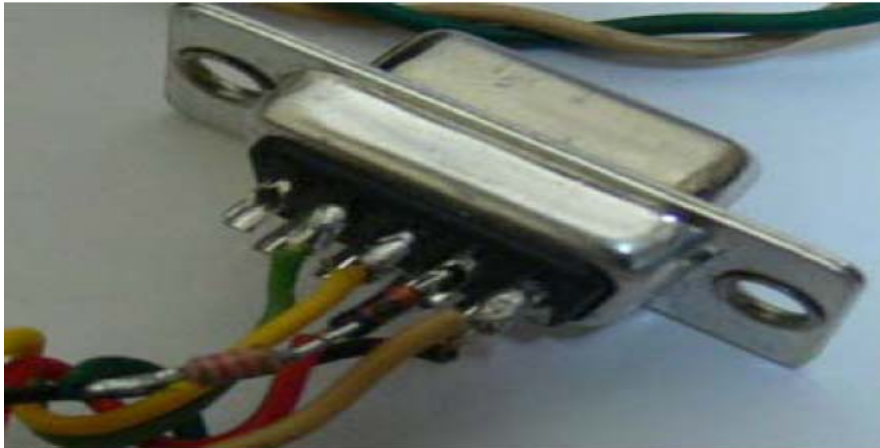
Figure 5. The diode connected on PIN-4
