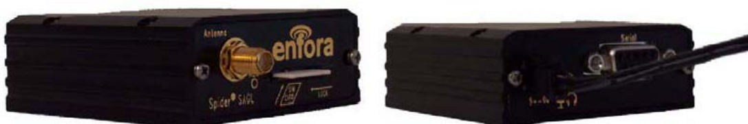
Figure 6. The GPRS modem used in Project.
