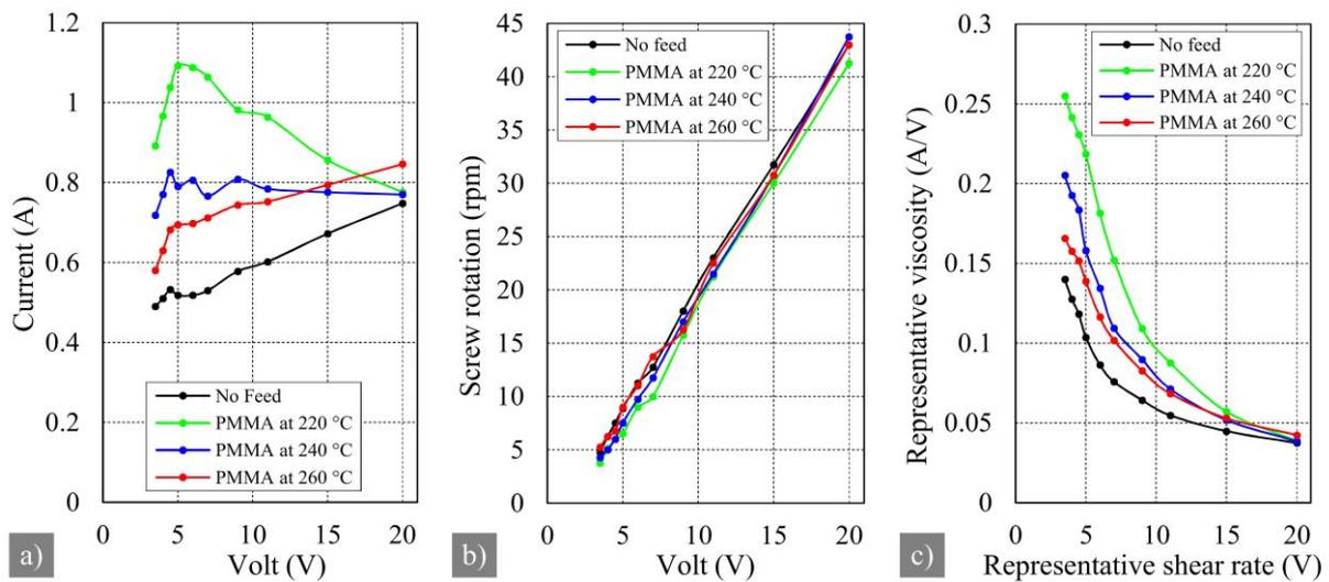
**Figure 10.** No-die case for PMMA a) current draw of the motor b) rpm vs. volt and c) representative viscosity plots of PMMA
