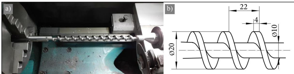
**Figure 5.** Screw details, *a)* a picture of produced screw on a regular lathe and *b)* technical drawing of the designed screw
