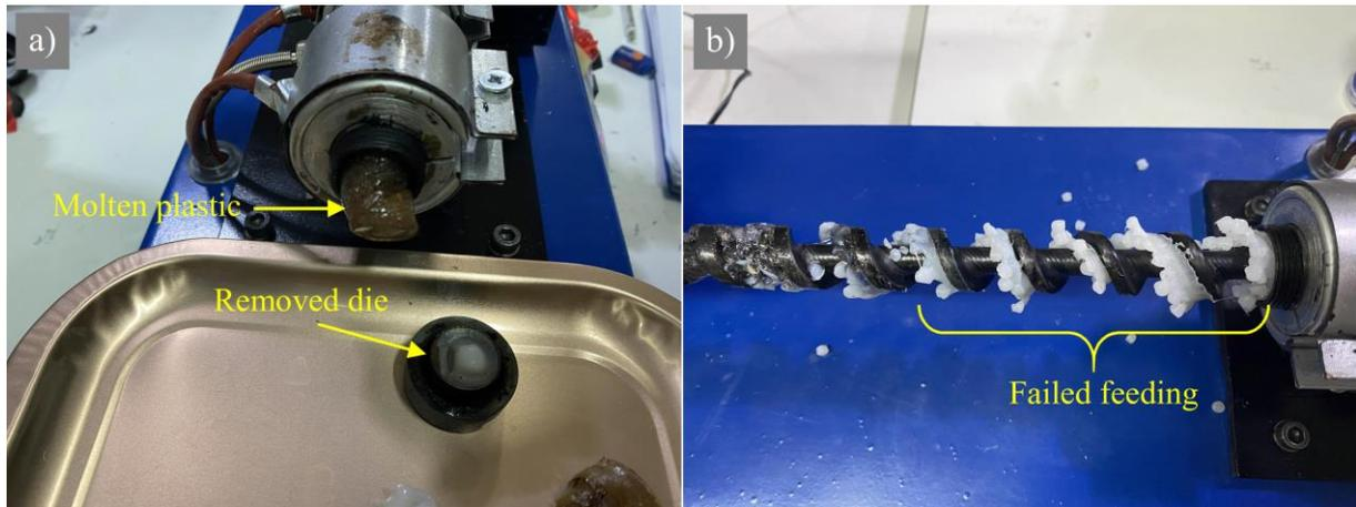
**Figure 7.** Experimental details of HDPE, **a)** removing the die and molten plastic picture and **b)** failed feeding of 260 °C case
