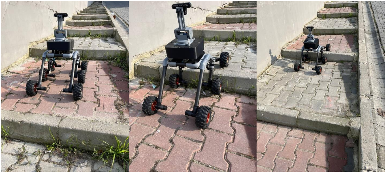
Figure 10. The robot was able to ascend stairs that ranged in height from 13 to 16 cm
