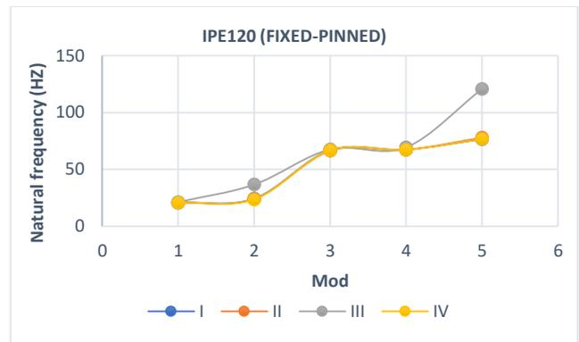
Fig. 15: Comparison of the natural frequencies for F-P with profile IPE 120 of castellated steel beams.
