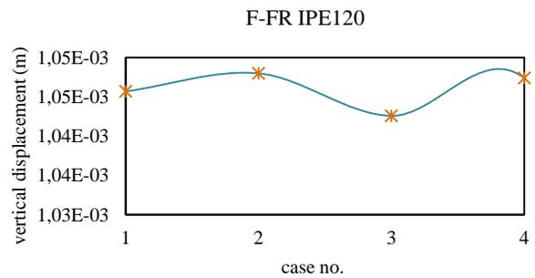
**Fig. 8:** Profil type – deflection curve for fixed –free castellated beam
