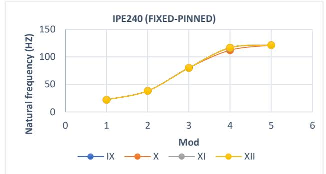
**Fig. 21:** Comparison of the natural frequencies for F-P with profile IPE 240 of castellated steel beams
