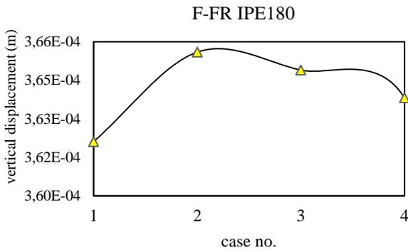
**Fig. 9:** Profil type – deflection curve for fixed –free castellated beam
