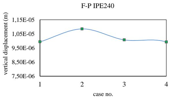
**Fig. 7:** Profil type – deflection curve for fixed –pinned castellated beam
