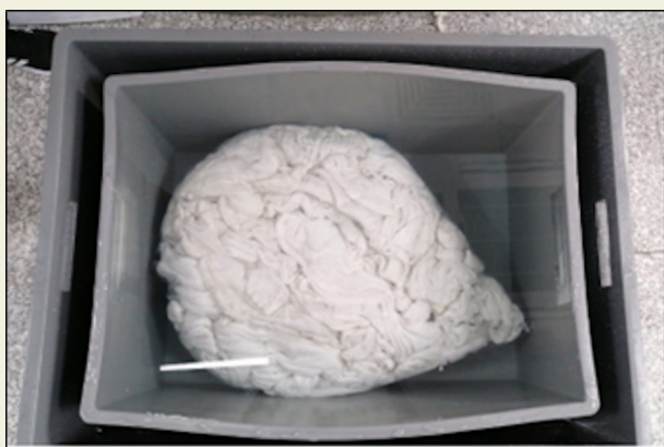
Figure 4. The volume of laundry measurement by water replacement
