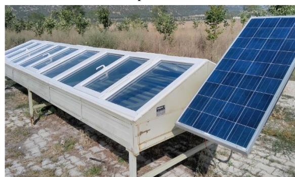
Figure 1 The experimental solar tunnel dryer
