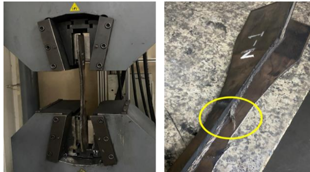
Figure 10. Breaking of specimen N-1 after tensile test.
