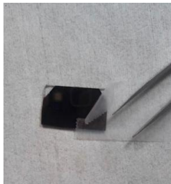
Figure 2. Scotch tape adhesion test of precursor Cu thin film deposited at 30 W.
