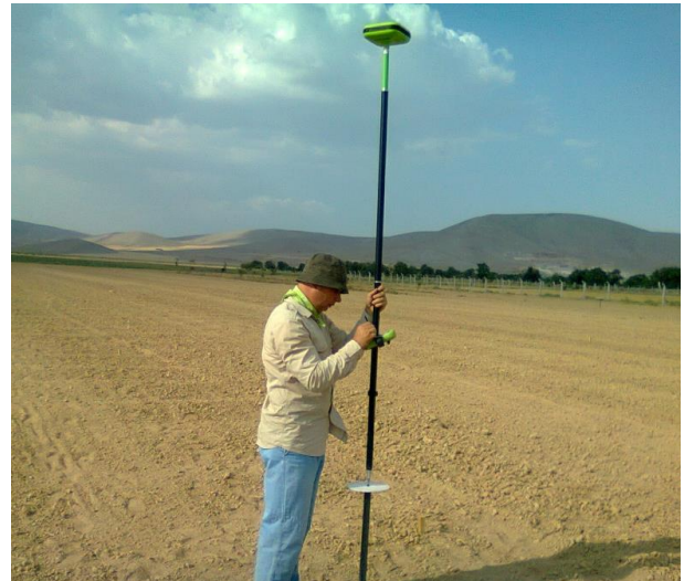
Figure 3 Coordinate points with a roving GPS tool
