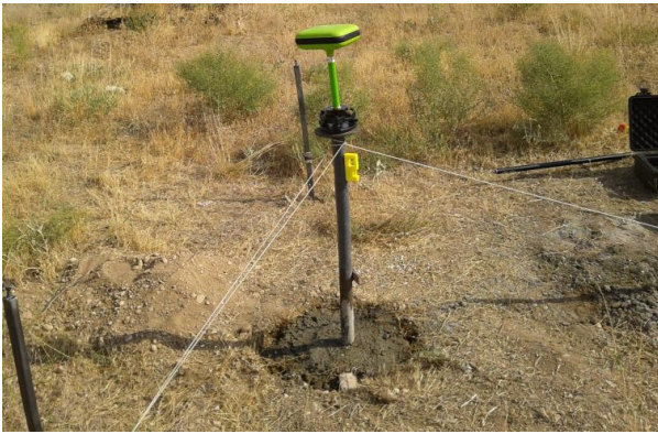
Figure 1 Fixed station established in work area
