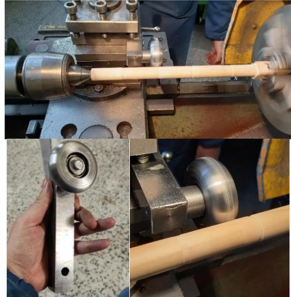
**Figure 5.** Densification of cylindrical parts with a spinning roller.
