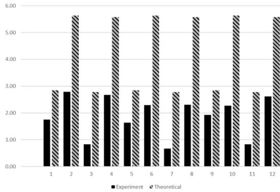
**Figure 7.** Experimental and theoretical % compression ratios according to the densification processes of the poplar wood.
