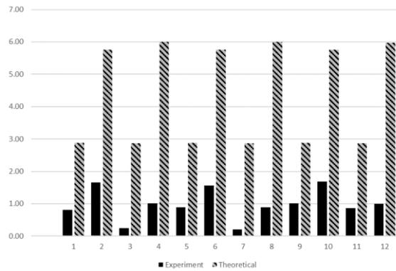
**Figure 8.** Experimental and theoretical % compression ratios according to the densification processes of the larch wood.
