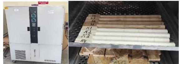
**Figure 2.** The position of the experimental specimens in the air-conditioned cabinet
