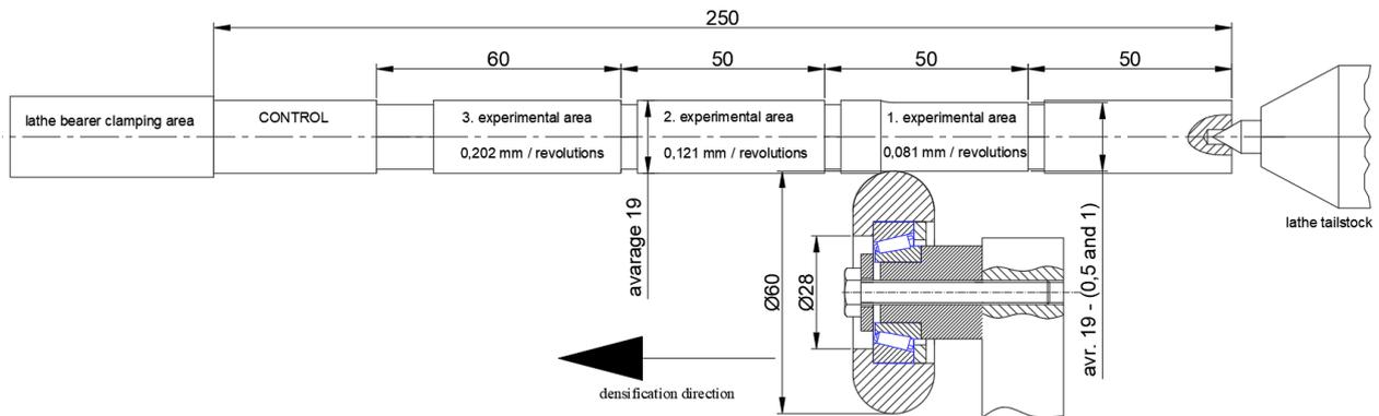
**Figure 3.** Schematic representation for surface densification process
