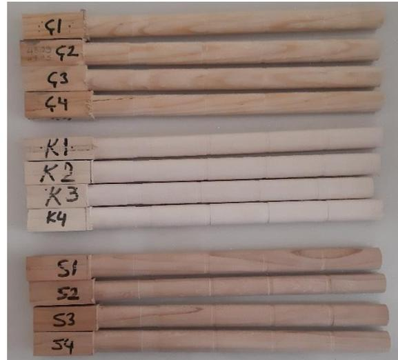
**Figure 1.** Test specimens before densification
