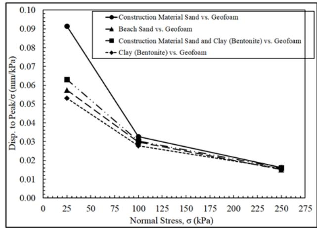
**Figure 10.** The variation in normalized interface engineering design parameters; normalized sensitivity (a) as well as normalized displacement to peak (b) as a function of normal stress
