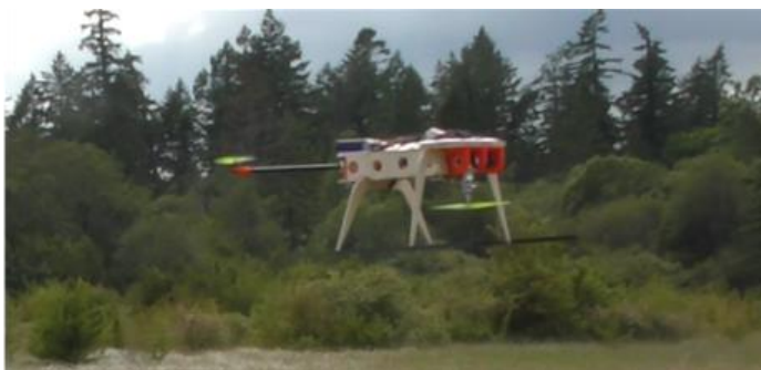
Fig. 7. Test tri-rotor during outdoor flight testing.
