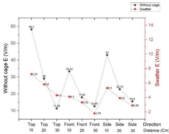
**Figure 13.** Electric fields versus the distance in cm from the shielding cage for the swatter (red) and shielding-free cases (black).
