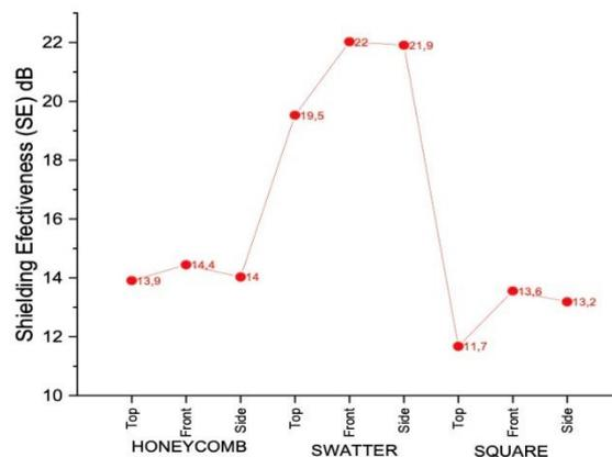
**Figure.** The shielding effectiveness of the plasma device for different shielding methods
