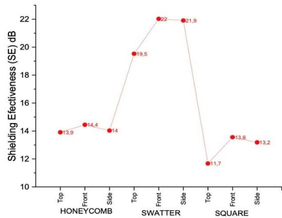
**Figure 15.** The shielding effectiveness of the plasma device for different shielding methods.
