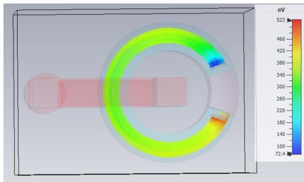
**Figure 4.** The simulation of electron trajectories due to the potential difference between the electrodes via the CST Particle Studio at  $p=1$  mbar;  $U=-500$  V.
