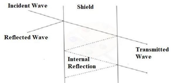
**Figure 1.** Attenuation of an electromagnetic wave by shielding technique.
