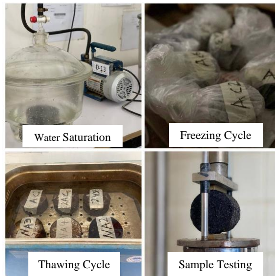
Figure 6. Moisture damage test
