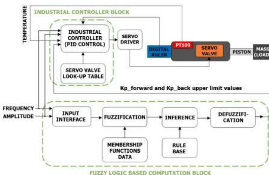
Figure 6. Block diagram of the control function of the hydraulic testing machine experimental setup
