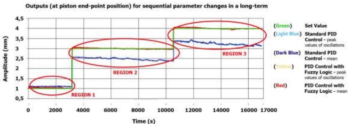
Figure 14. Comparison of output data obtained against sequential parameter changes in a long-term (~300 min) test (frequency input 4 Hz, amplitude input ±1, ±3, and ±4 mm)
