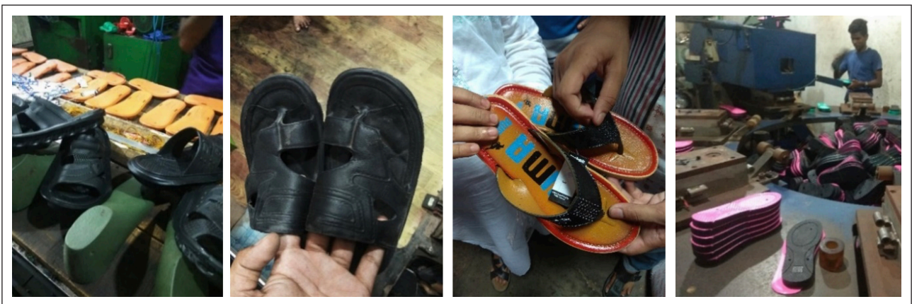
Figure 16. Second grade shoes in black hue, third grade shoes in black hue, painted third grade shoes and mixed grade shoe soles where the pink part is new and the black part is recycled (left to right).
