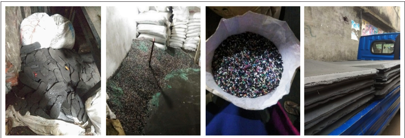
Figure 15. Old shoes for recycling, crushed chips of old shoes and recycled sheets (left to right).
