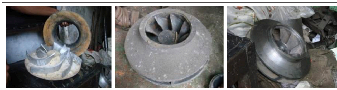
Figure 3. Dice making, molded metal section and finished product (left to right).
