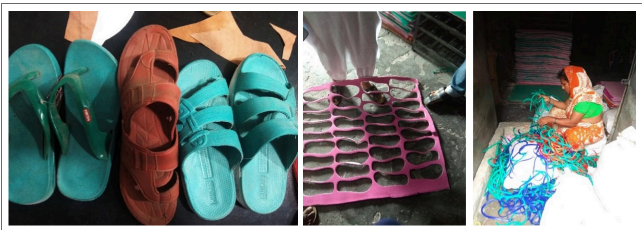
Figure 14. First grade (newly produced) shoes, left over cuts of soles to be reused in the production (left to right).
