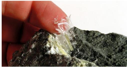
**Figure 1.** Asbestos in a Construction Material (Çember, 2022).
