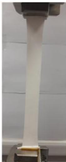
Figure 2.4 Connection of the samples to the pulling test device
