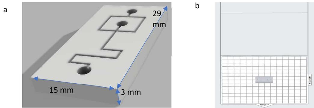
**Figure 1** (a) View of the microchannel in CAD file (b) microchannel directly placed over the build platform in Preform software.
