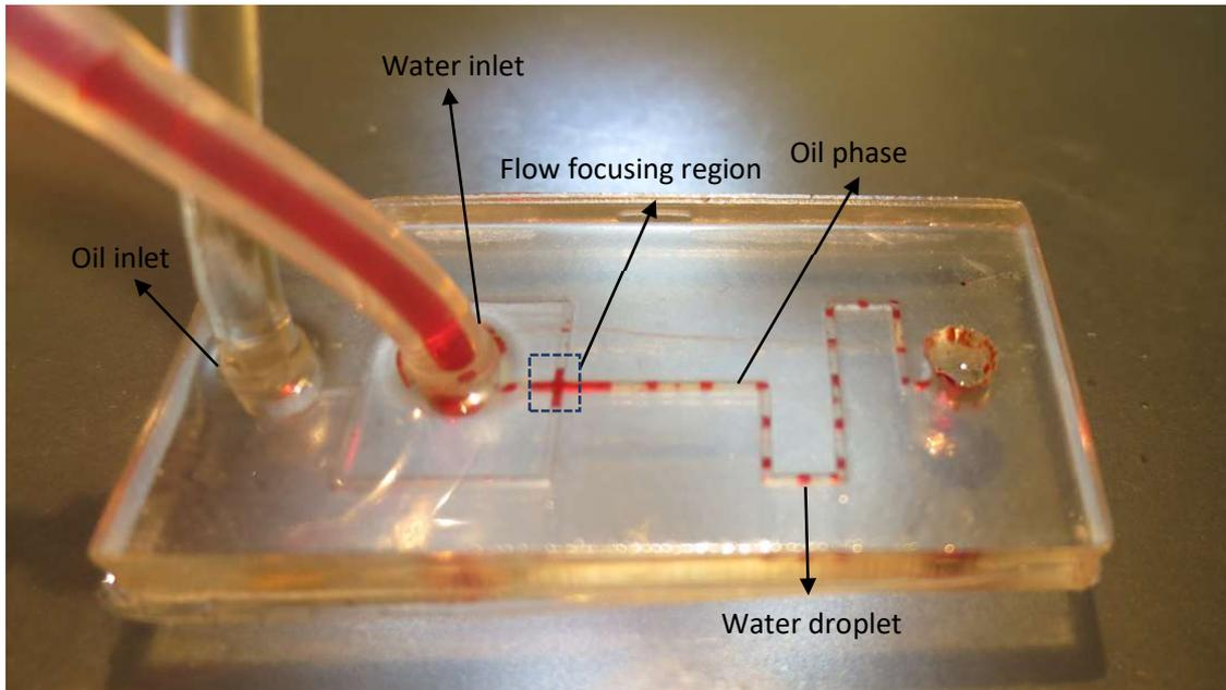
Figure 2 3D printed microfluidic chip with fluidic connection
