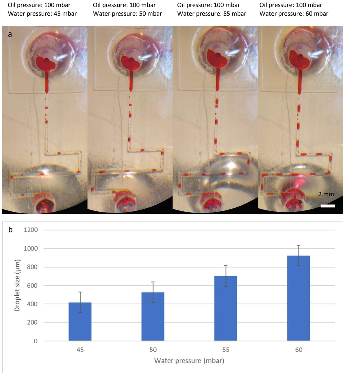
**Figure 3** Water in oil droplets in a microchannel **(a)** Microscope photo microdroplets inside the channel for several water pressures. **(b)** Droplet size across water pressure.
