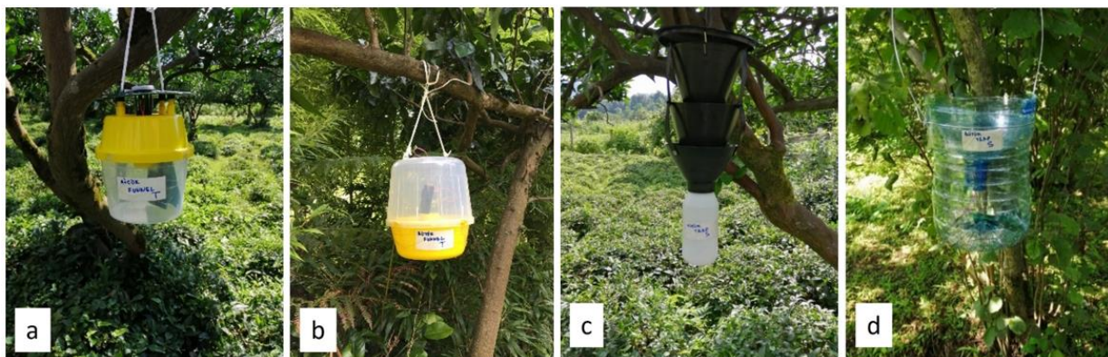
Figure 1. Different traps types: (a) Small funnel trap; (b) McPhail trap; (c) Multi funnel trap; (d) Big funnel trap.
