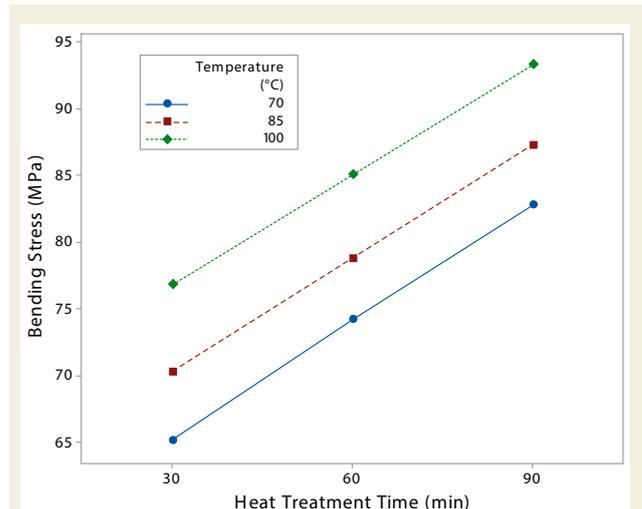
Figure 9. Effect of heat treatment on bending stress
