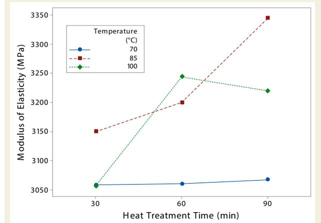
Figure 5. Effect of heating treatment on mudulus of elasticity
