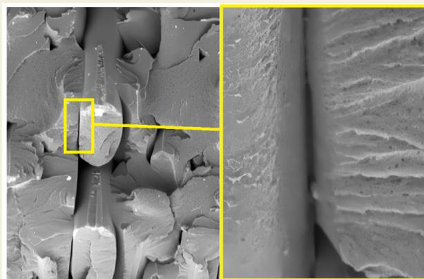
Figure 11. PLA tensile test fracture surface without annealing
