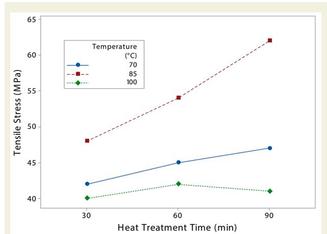
Figure 4. Effect of heat treatment on tensile stress
