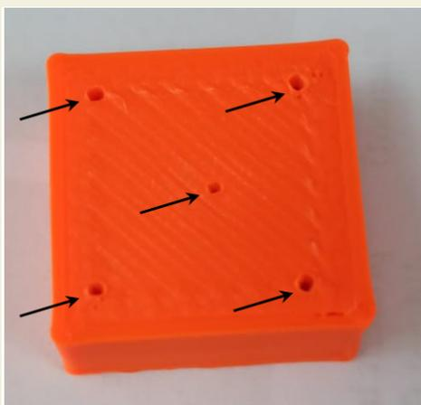
Figure 7. Appearance of needle marks on the sample
