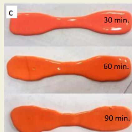
Figure 2. a) Some of the test samples b) Annealing in the furnace c) Samples melted at 155 °C
