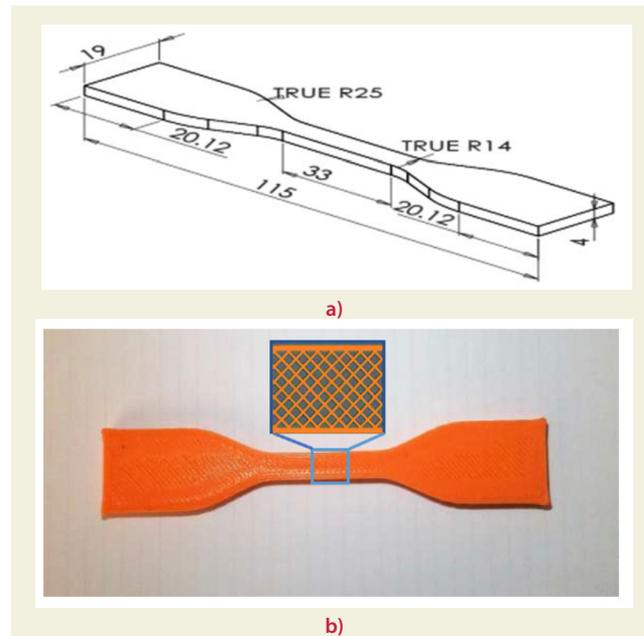
Figure 1. a) ASTM D638 Type-4 tensile specimen standard dimensions [12], b) Printed specimen
