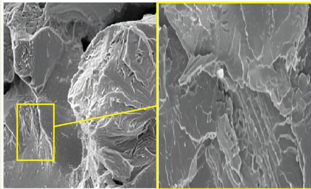
Figure 10. PLA tensile test fracture surface annealed at 85 °C
