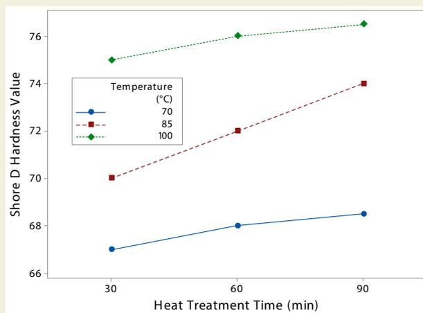
Figure 8. Effect of heat treatment on Shore D hardness value
