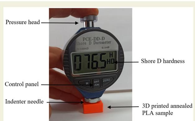
Figure 6. Hardness measurement with durometer
