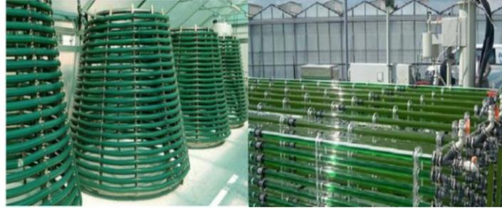
**Figure 5.** Horizontal (flat) production system in photobioreactor (Gezici, 2012).
