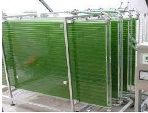
**Figure 4.** Flat-panel photobioreactor production system (Kükdamar & Tokuç 2015).
