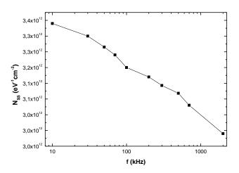
Figure 5. The variation of the  $N_{ss}$ , for the Al/TiO<sub>2</sub>/p-Si MIS structure as a function of the frequency at room temperature.
