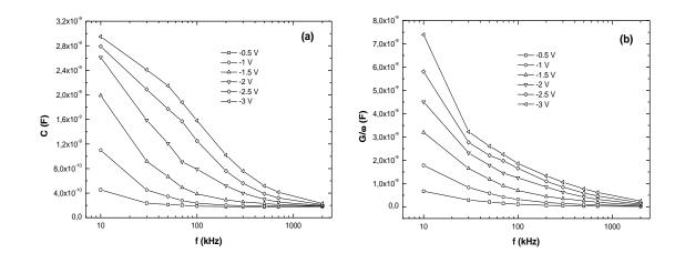
Fig. 2. (a) The capacitance-frequency and (b) conductance-frequency characteristics of Al/TiO2/p-Si MIS structure for various reverse bias at room temperature.
