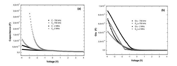
Fig. 4. The voltage dependent plot of the corrected the high frequencies (a) capacitance and (b) conductance curves at room temperature.
