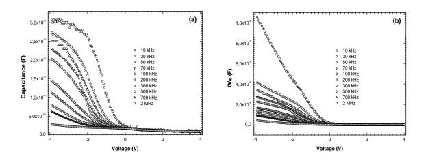
Figure 1. The frequency dependent plots of (a) the capacitance-voltage and (b) conductance-voltage characteristics of Al/TiO2/p-Si MIS structure at room temperature.
