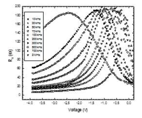
Fig. 3. The variation of the series resistance as a function of voltage for various frequencies of Al/TiO2/p-Si MIS structure at room temperature.
