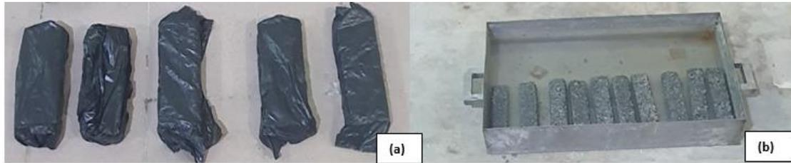
Figure 2: (a) Specimens of autogenous shrinkage; (b) Specimens of expansion.
