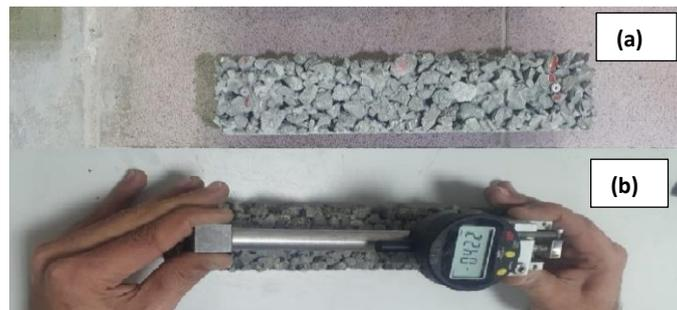
**Figure 1:** (a) Sample with two demec points; (b) Dial gauge machine.
