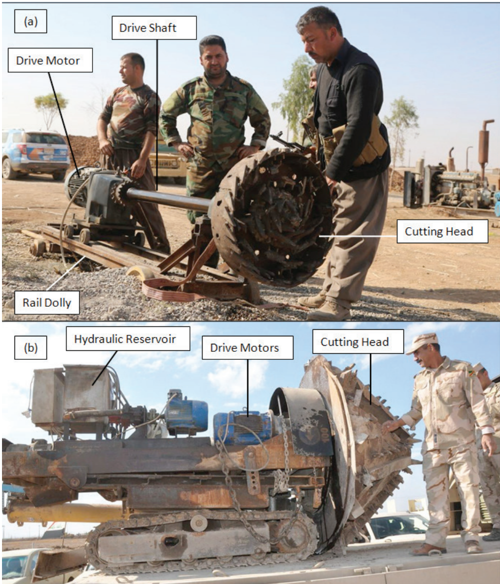
Figure 5. (a). View of the front of a captured ISTBM showing the cutting head with Peshmerga fighters for scale 125 . (b). Side view of a captured ITTBM on a flat bed truck with Iraqi soldiers for scale 126 .
