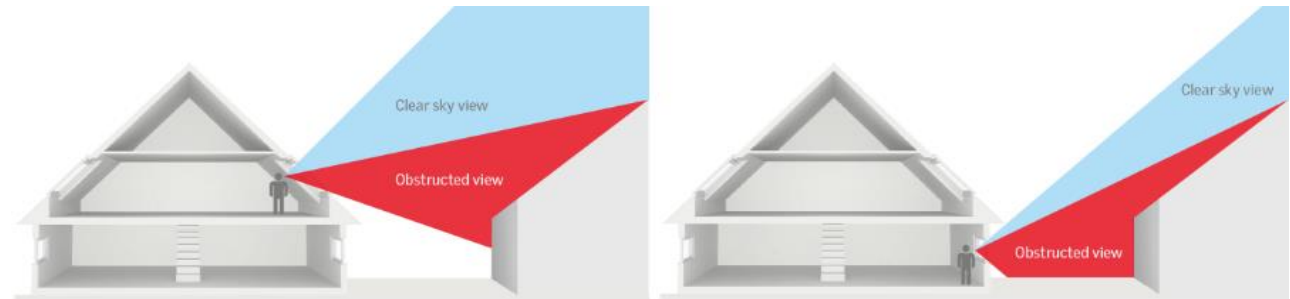
Figure 6. Components of view-roof window and view-facade window situations [40]
