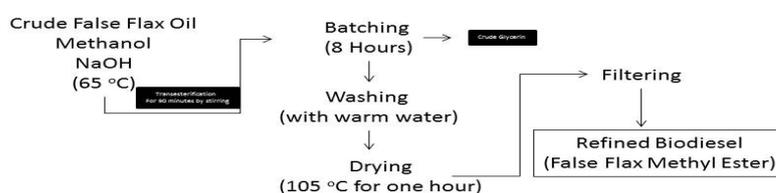
Figure 1: Biodiesel production flow diagram
