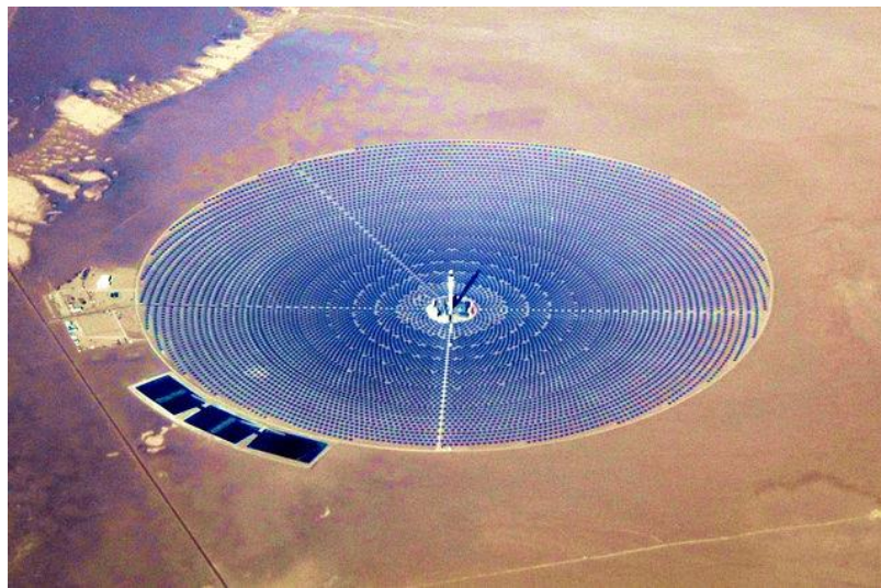
Figure 6. A solar power tower covering an area of 1.21 km 2 and concentrating light using 10,000 mirrored heliostats [3].
