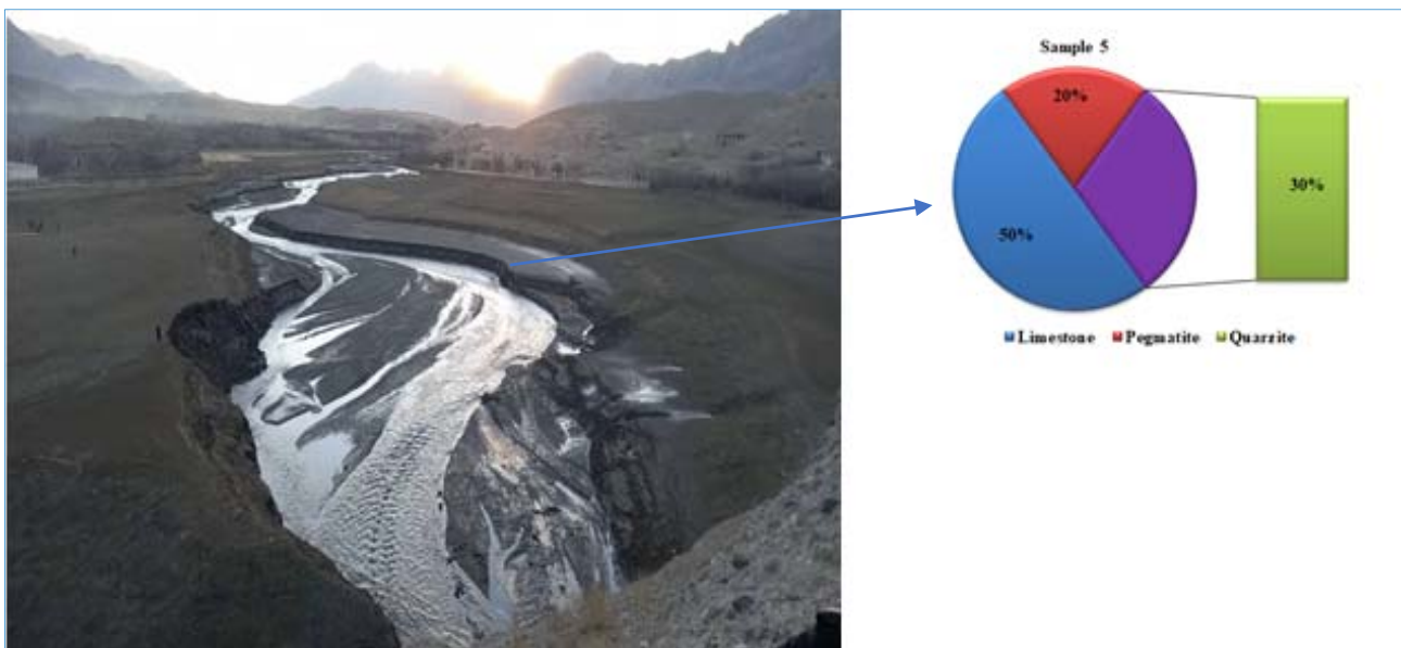
Fig. 16. Gravel analysis in point 5 and find different types of rocks in sediments
