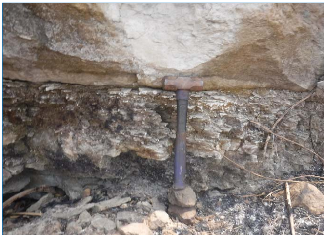
Fig. 9. Shows closed-up view of sharp boundary between hummocky cross stratified sandstone and the underlying Eze-Aku shale. The length of hammer is 34 cm
