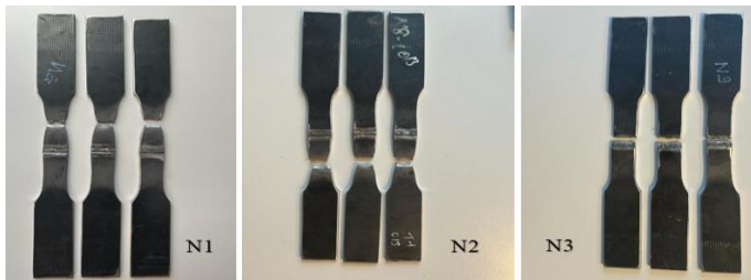
Fig.5 MAG welded samples' photographs after tensile test
