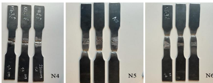
Fig.6 SMAW welded samples' photographs after tensile test
