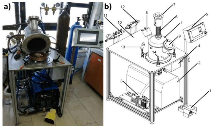
**Figure 1.** Vacuum arc melting experimental setup a) Photograph image, b) schematic picture (1: Sleeve, 2: Power unit, 3: Vacuum pump, 4: Control panel, 5: Control unit, 6: Bellows, 7: Electrode movement wheel, 8: Lighting window, 9: Observation window, 10: Tray, 11: Water inlet control circuit, 12: Water outlet control circuit, 13: Supporting apparatus, 14: Stabilizing hinge, 15: Arc control pedal)
