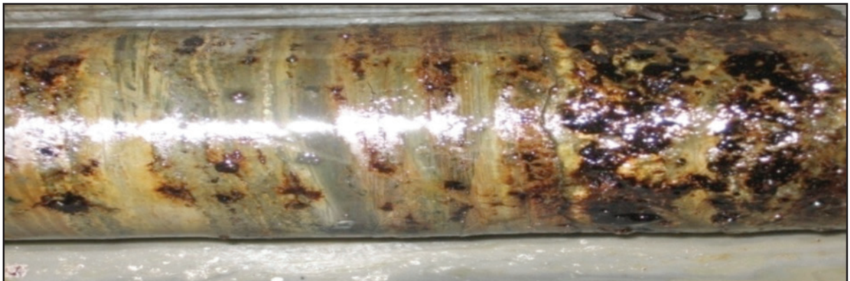
Figure 8- Bituminous shale core with liquid petroleum indications cut at 462 m in Yeniköy drilling KEY-08/02 (x: 4176100, y: 613550).
