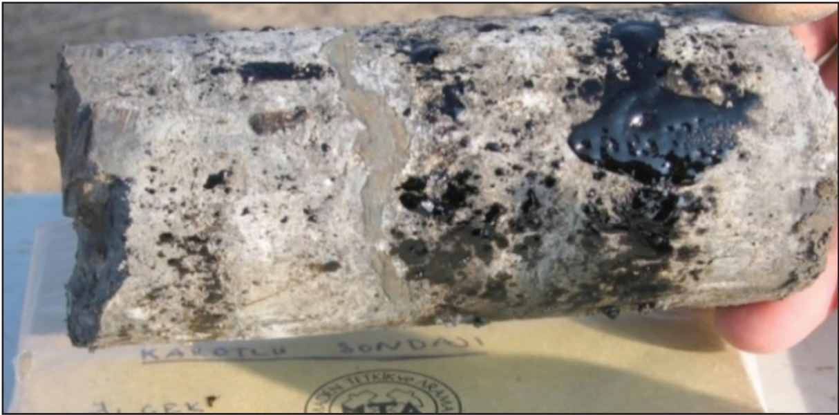
Figure 9- Liquid petroleum infilling the pores of dolomites cut in Yeniköy drill KEY-08/04 (371 m).
