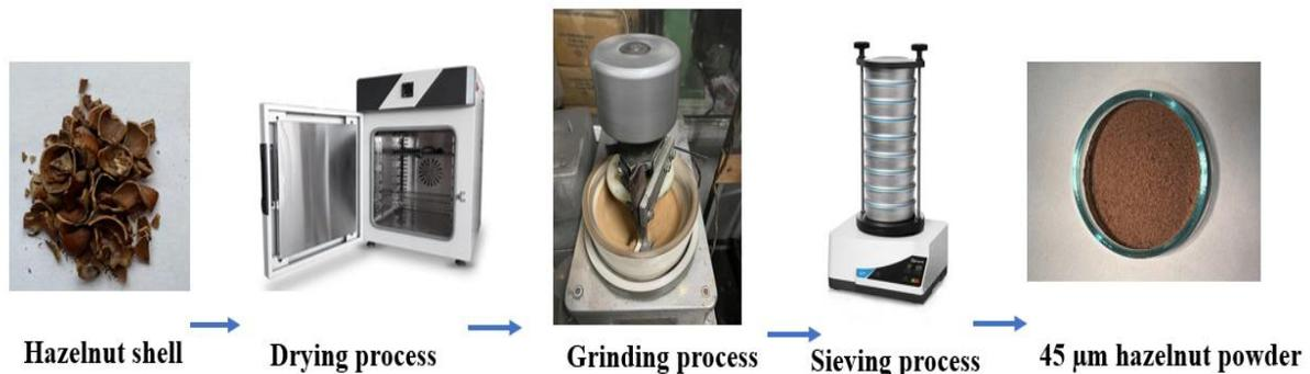
**Figure 4.** Hazelnut powder grinding process sequence
