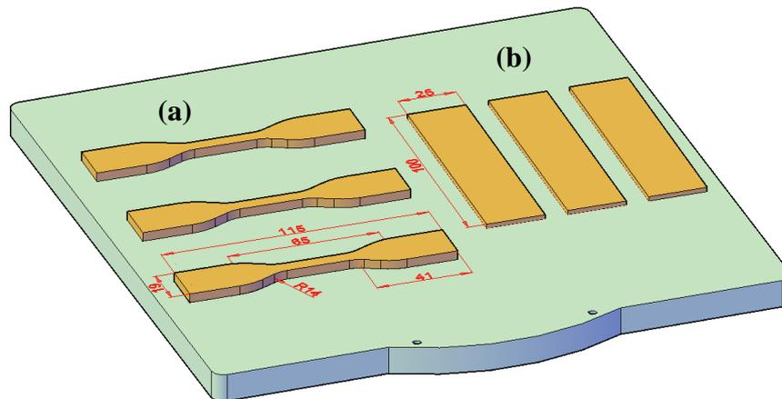
**Figure 2.** Tensile specimens and bonding plates dimensions (mm)
