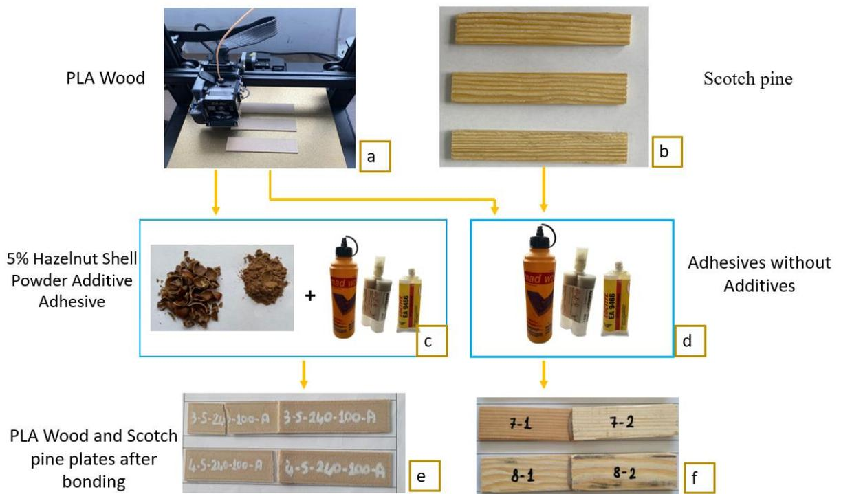
**Figure 1.** Flowchart of the adhesive bonding process
