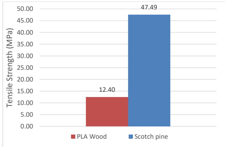
**Figure 5.** Average tensile strength values of test specimens
