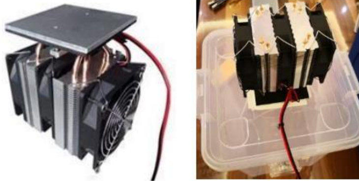
Figure 7. Thermoelectric cooler module block and water tank with copper, aluminum cooler, and fan circulation used in the system (Özcan, Çelebi & Arpacioğlu, 2022)
