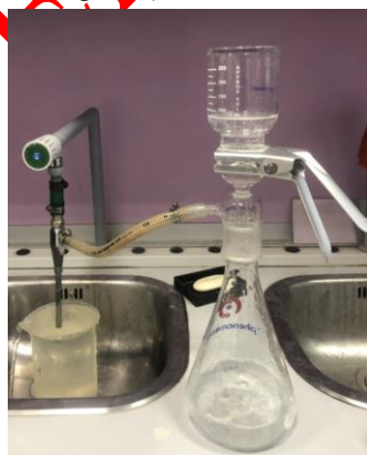
Figure 1. Filtration process for separation of MFs.
